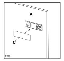
Open the appliance door and the furniture door at  $90^{\circ}$ . Insert the small square (B) into guide (A). Put together the appliance door and the furniture door and mark the holes as indicated in the figure. Remove the squares and drill holes with  $\emptyset$  2 mm at 8 mm from the outer edge of the door. Place the small square on the guide again and fix it with the screws supplied.
